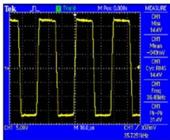
Voltage across the capacitor is approximately  $150V_{RMS}$
