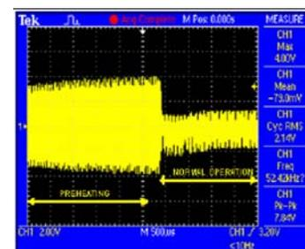
Generally, the capacitance value of the pre-heat capacitor is more than that of the striking capacitor. For example, if the value for C6 is 0.0047-0.01 $\mu\text{f}$  then C7 will be 0.0018-0.0068 $\mu\text{f}$ .
