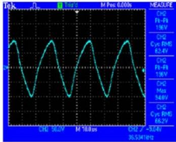
After preheating operation the lamp goes in to normal operation.  $V_{RMS}$  across the striking capacitor during normal operation is 65 V.
