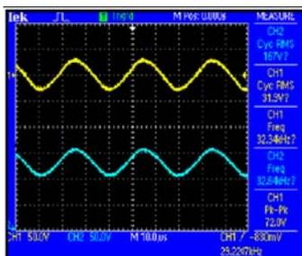
Here AC voltage super imposed on DC voltage.
