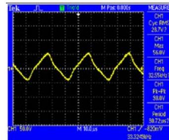
In the pre-heat function, the load across the striking capacitor is shared by the pre-heat capacitor.
