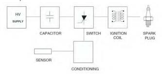
The HV supply for the CDI is is supplied by a DC/DC converter. This stage provides 400V from the 12V battery. The value of capacitor generally lies between 0.47 and 2.2 $\mu$ F. This capacitor is used to store the charge from the HV supply.
