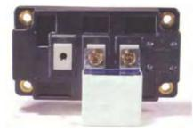
The acceptable amount of overshoot voltage is determined by the maximum DC voltage that an inverter power circuit is subject to and the IGBT voltage ratings. The peak current to turn off under a fault condition can be as high as 6 - 10 times the device current rating. This peak current under the fault condition will proportionally increase the overshoot voltage.
