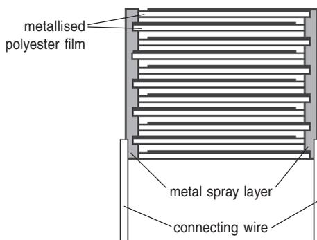
Here instead of using 6 micron thick foil, the plastic film (dielectric) is coated with either aluminium or zinc alloy material. Metal particles are vacuum deposited directly on to the plastic films. Thickness of the metallisation is approximately 30 nm. This drastic reduction in thickness of electrodes leads to the relatively smaller dimensions for metallised film capacitors.
