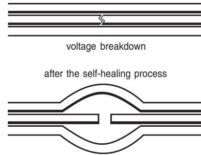
This dielectric puncture is in fact a momentary short-circuit (lasting a few microseconds) and hence the capacitor regains its full operation immediately. There is, however, a slight drop in the capacitance value, on account of the isolated area.
