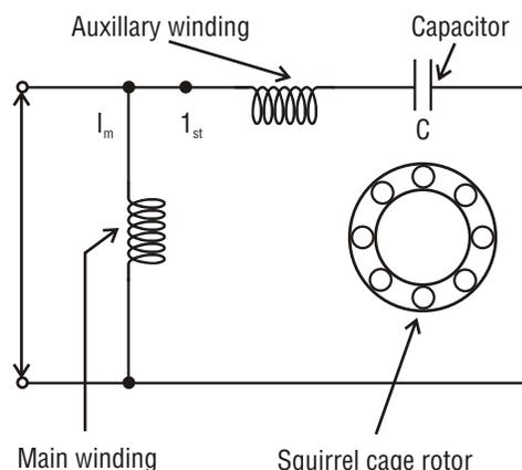
current of near 90°. Once started the auxiliary winding is optional. The auxiliary winding of a permanent-split capacitor motor has a capacitor in series with it during starting and running.
